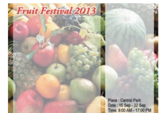
Processing with CPSI The translucent images are incorrectly reproduced. The output is not what the user intended for.
